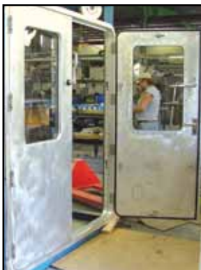
Quick-acting version, Active panel open, Unpainted
